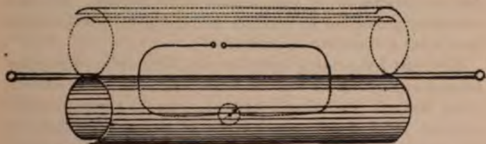
Fig. 80. EFFECT OF ENCLOSURE IN PREVENTING SPARKS.
